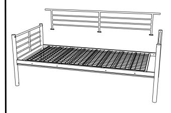
Insert #5 Side Rail B into location hole on #3 Top Frame
