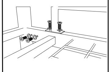
Use **Bolt C** and **Washer A** to secure Base and Rails.
